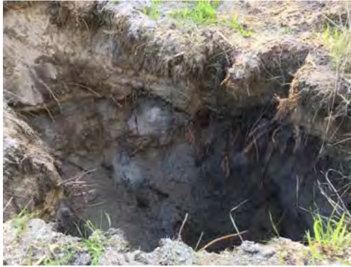
Plate 5: Uncontrolled Fill and topsoil overlying natural Sand within test pit (TP 5)
