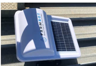
Farm bot positioned on top of tank
