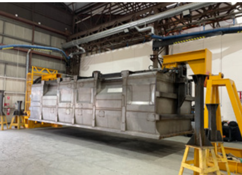
Iron ore rail wagon being manufactured.
