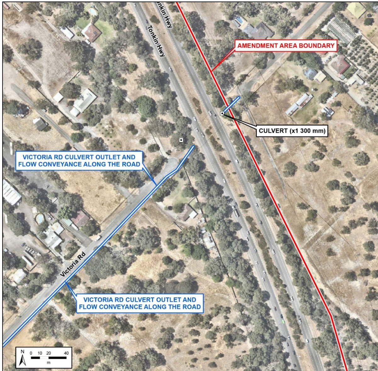
Figure 5-18: Surface water flow path conveyed via the Victoria Road culvert.
