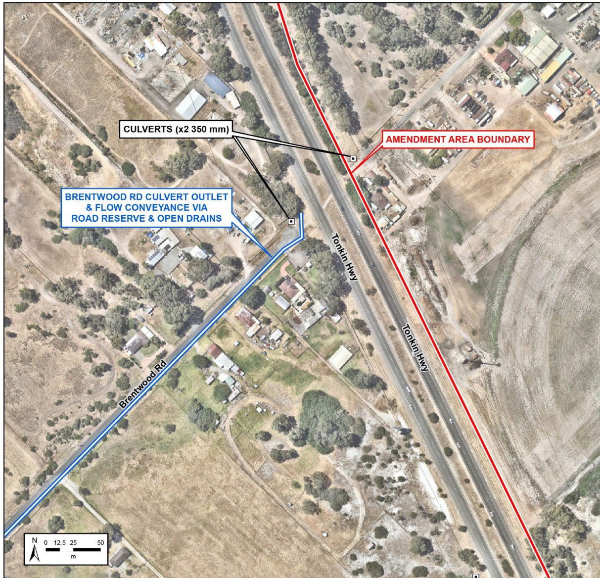
Figure 5-19: Surface water flow path conveyed via the Brentwood Road culverts.
