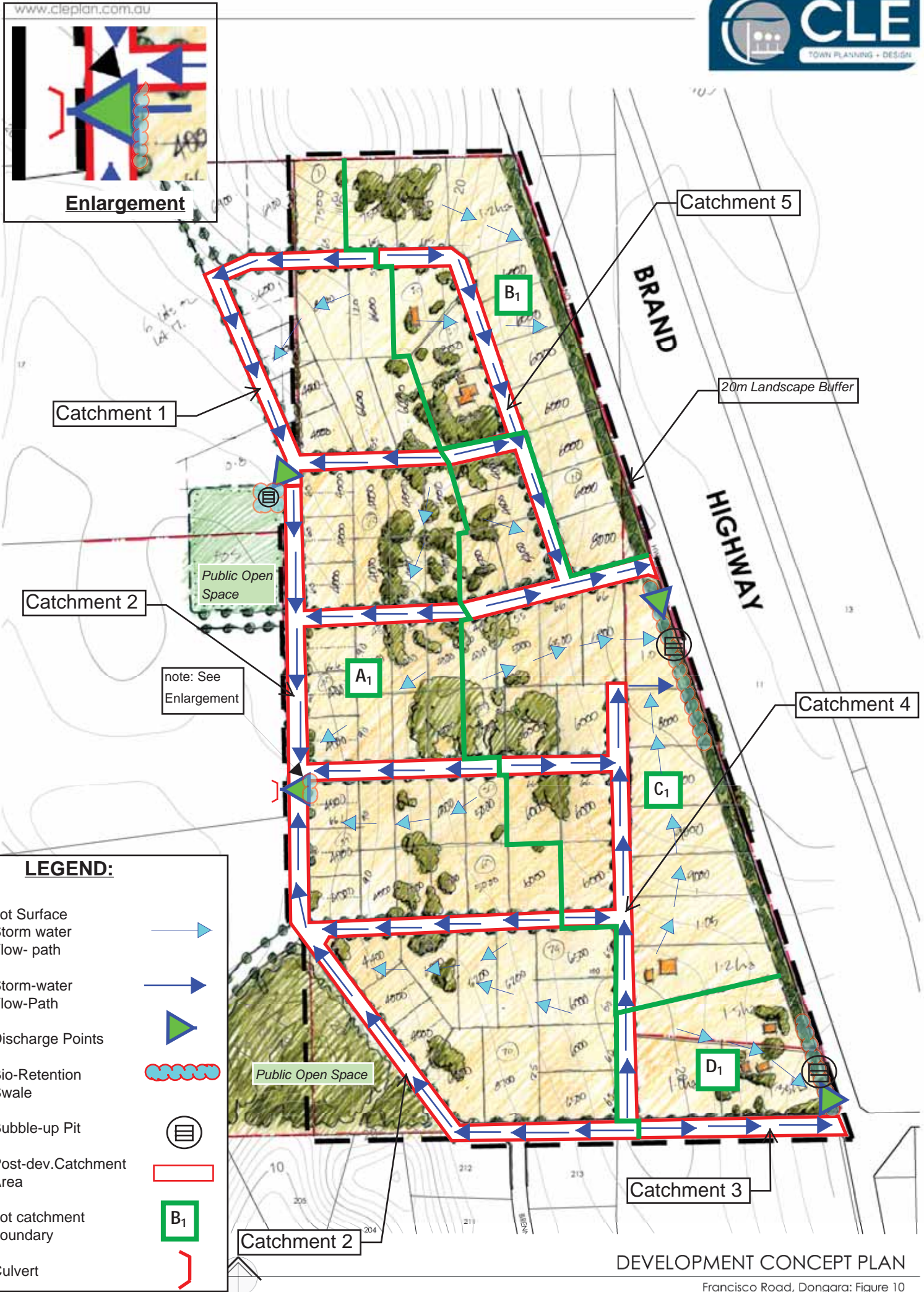
Figure 7: Post-development Surface Runoff and Disposal
