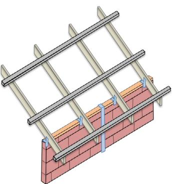
Figure 04 Tie-down strap over tie-down/cavity batten
