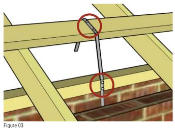
This acts as a two nail connection to either the over-batten or wall plate
