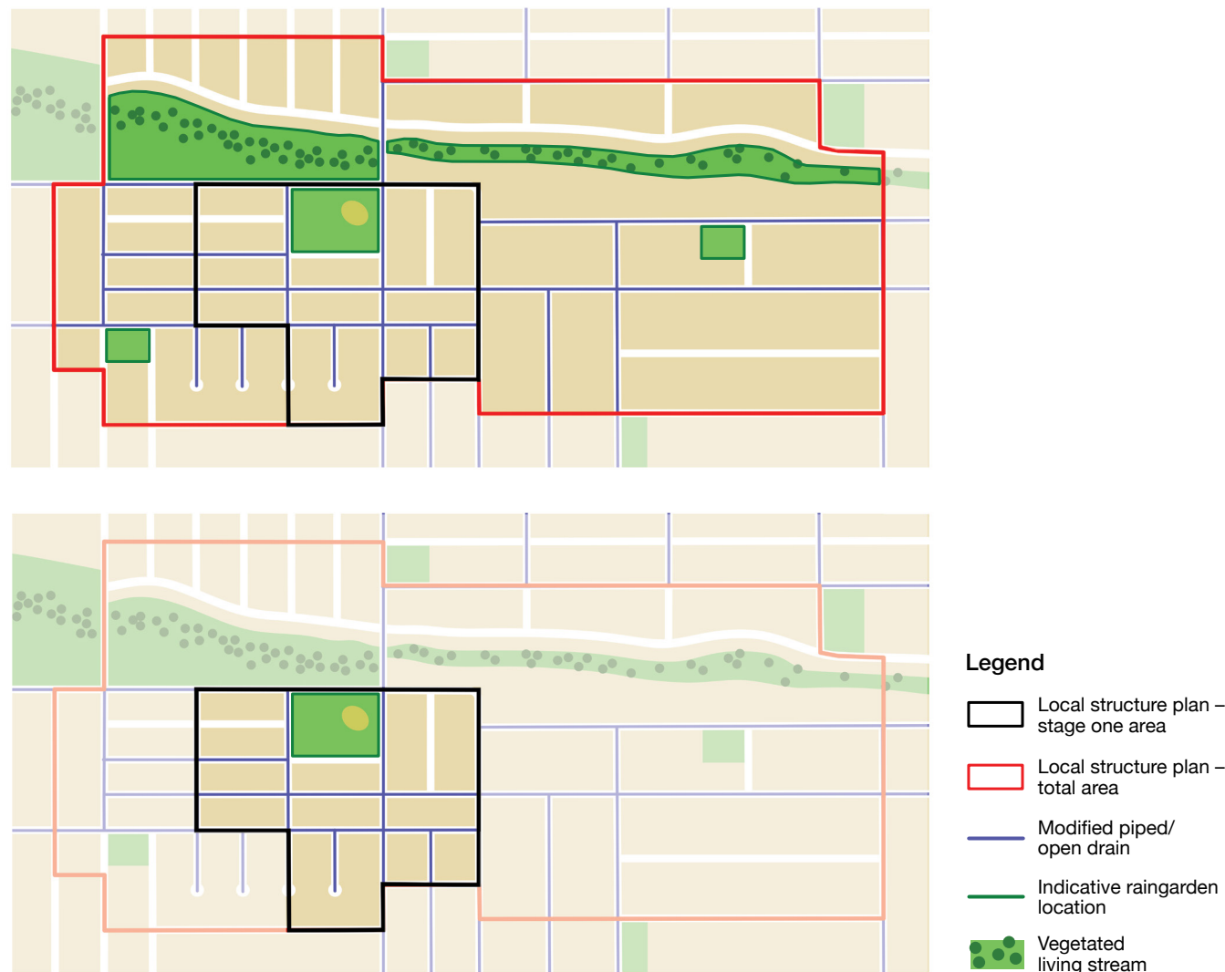
Figure 4: The ultimate (top) and interim (bottom) stormwater management system layouts for this site show an increased level of detail for the initial stages of a proposed development
