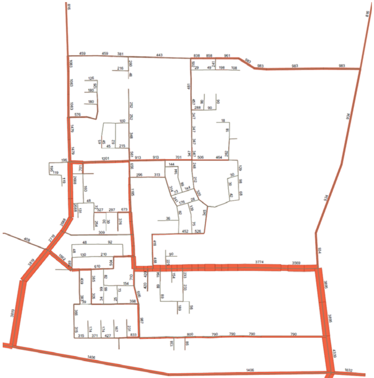
Figure C1. Daily traffic generated by medium term development in Dayton (short-term road network scenario 1 – with access to West Swan Road via Coast Road and Victoria Road; no Lord St extension south of Reid Hwy)
