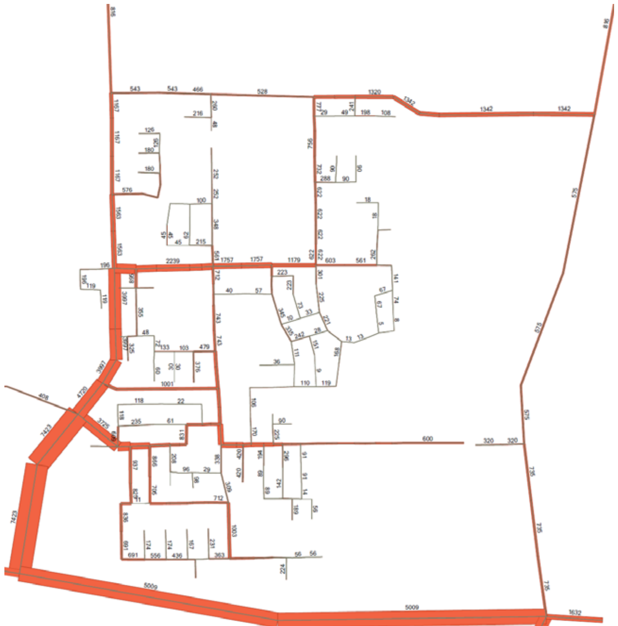
Figure C2. Daily traffic generated by medium term development in Dayton (short-term road network scenario 2 – no access to West Swan Road via Coast Road and Victoria Road; no Lord St extension south of Reid Hwy)
