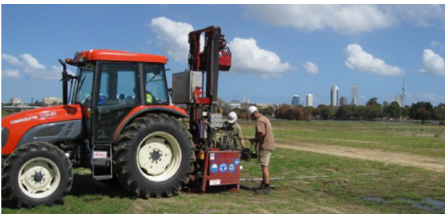
Tractor-mounted sonic drill rig taking core samples as part of the department's ASS mapping program
