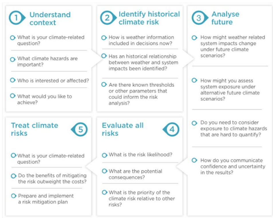
Figure 8 Climate risk assessment framework from the electricity sector climate information user guide
