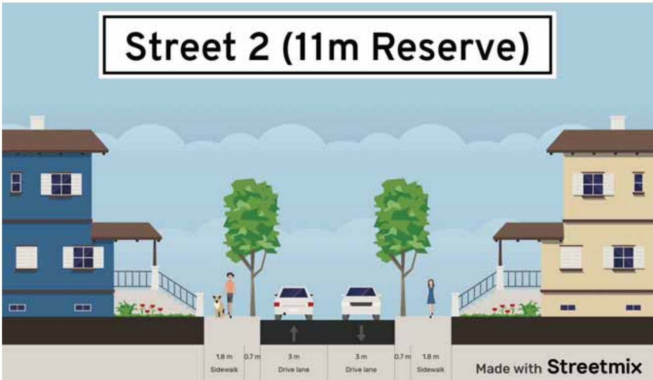
Figure 4-3: Cross-Section for 11m Street 2
