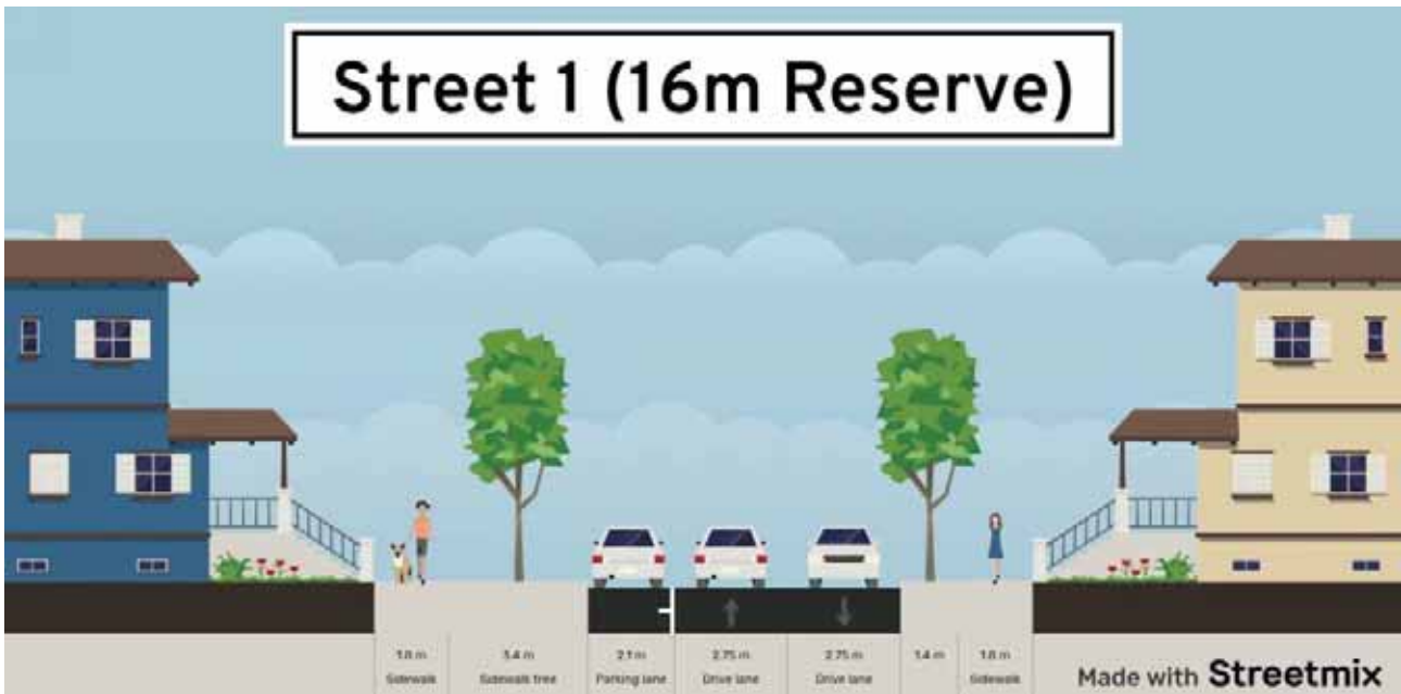
Figure 4-2: Cross-Section for 16m Street 1
