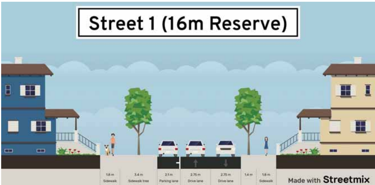
Figure 4-2: Cross-Section for 16m Street 1
