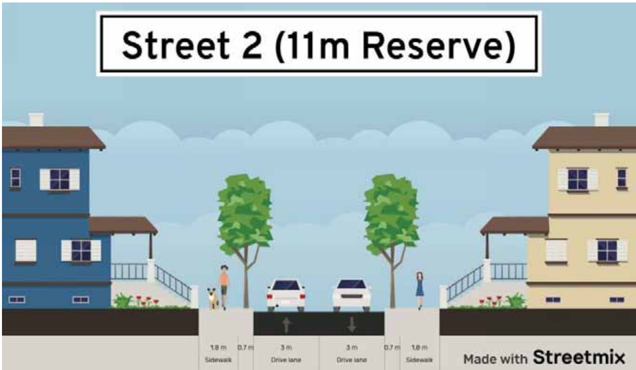
Figure 4-3: Cross-Section for 11m Street 2
