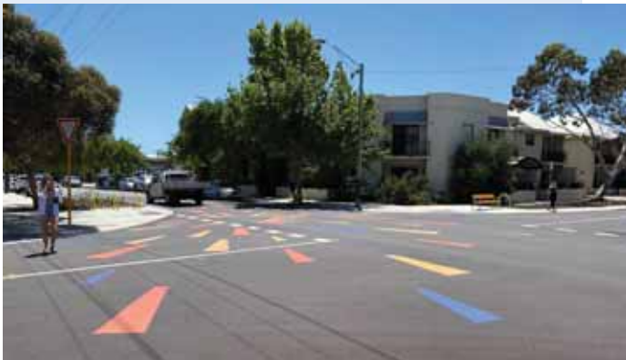
Image 6: A standard-width intersection modified to be raised, achieving continuous footpaths with no level change for pedestrians (South Fremantle)
