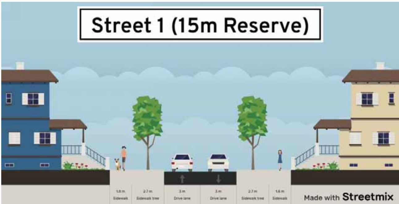
Figure 4-1: Cross-Section for 15m Street 1
