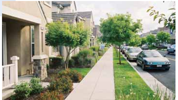
Image 5: A street with a footpath uninterrupted by crossovers, creating more landscaping space and better safety for pedestrians (San Mateo, California)
