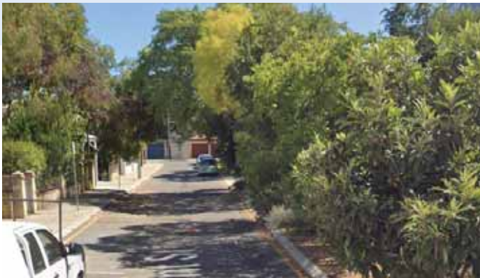
Image 4: A narrow street with two-way carriageway (6m-wide) that narrows at single-lane points to enable on-street parking and slow-moving traffic to pass (Fremantle)
