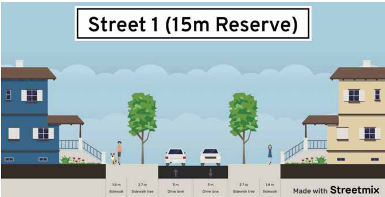
Figure 4-1: Cross-Section for 15m Street 1
