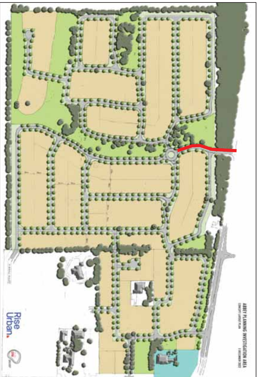
Figure 4-3: Road Hierarchy within Development (Access Street B in red; Access Street D all others)
