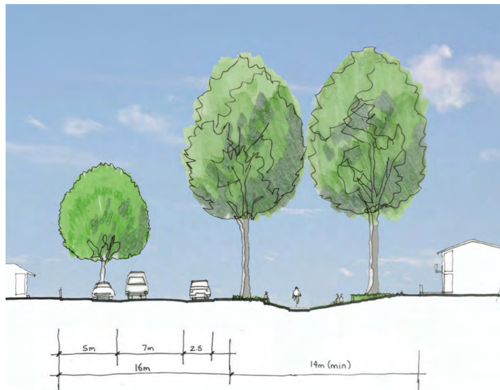
FIGURE 27 - CROSS-SECTION OF THE TAMALA PARK WEST OF CONNOLLY DRIVE ADJACENT A NEIGHBOURHOOD ACTIVITY CENTRE OR OTHER ACTIVITY NODE.
