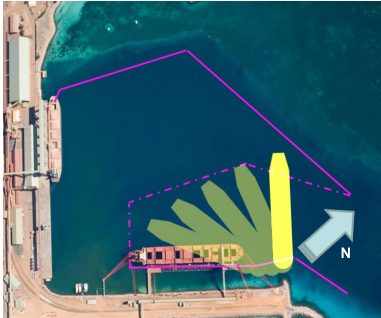
Figure 6: Movement of ship towards the north once the lines holding the ship break, blocking the inner channel for the MTE scenario. Image supplied by Southern Ports Authority – Port of Esperance.
