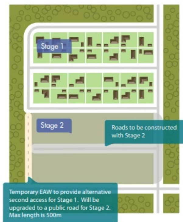
Figure 22: Example of an emergency access way
