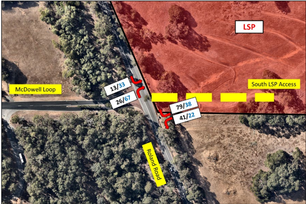
Figure 18: Estimated traffic flows at Roland Rd/McDowell Loop/South LSP Access Intersection – AM/PM Peak (Stage 1)
