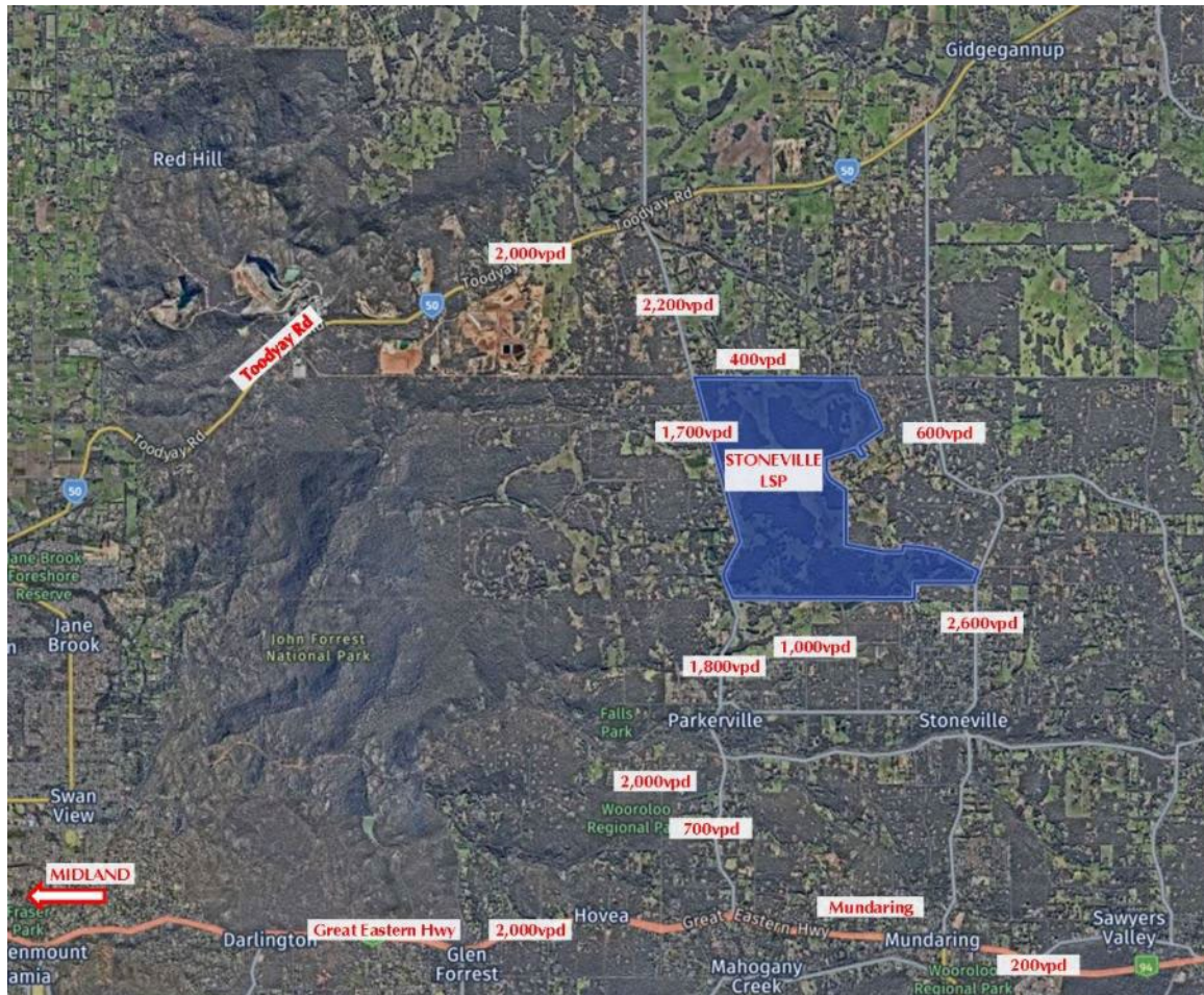
Figure 32: Projected additional daily traffic volumes from the LSP on regional roads with full North Stoneville LSP build-out
