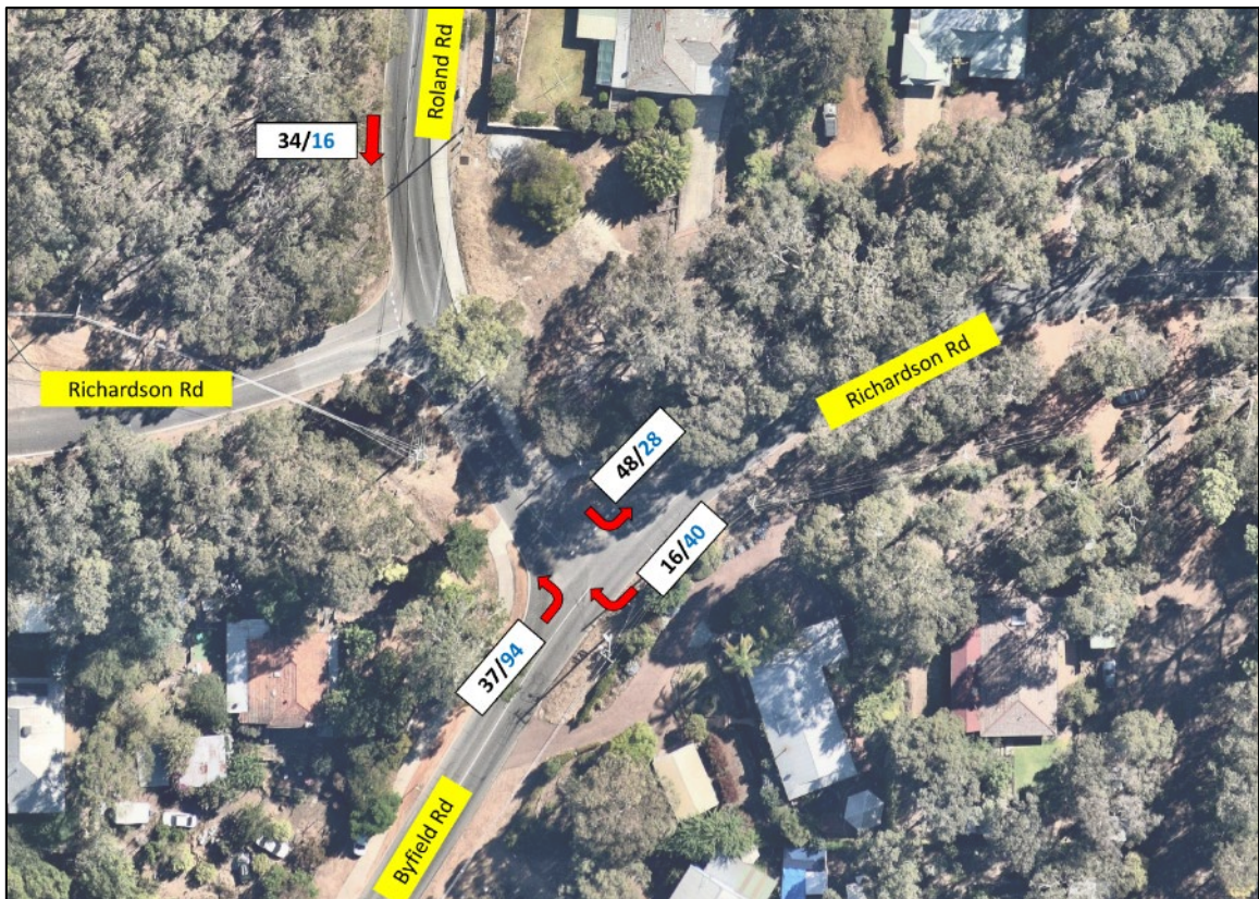
Figure 19: Estimated traffic flows at Roland Rd/Richardson Rd/Byfield Rd Intersection – AM/PM Peak (Stage 1)
