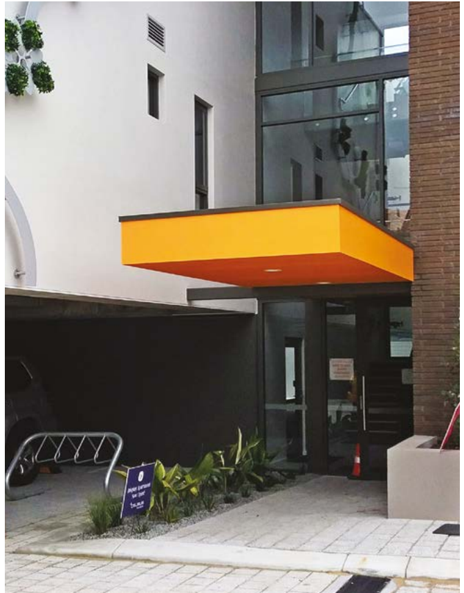
Photo 3.9e Convenient, secure and undercover parking for bicycles is located next to the entrance of this apartment block.
