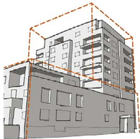
Figure 2.1a The final built form will usually differ significantly from the building envelope, due to plot ratio constraint as well as necessary articulation of building for light, ventilation, open spaces and circulation.
