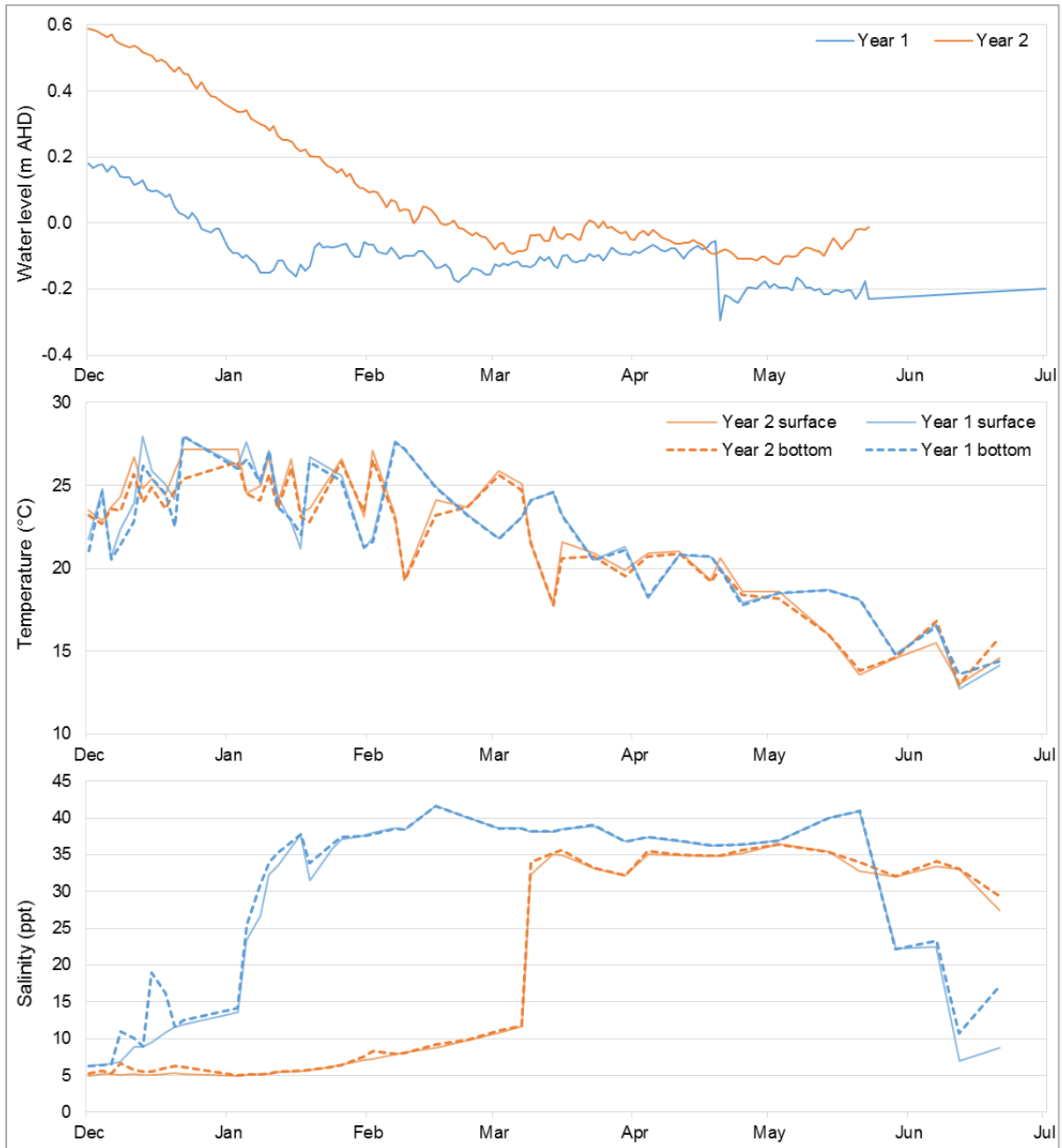
Figure 5 Water levels (m AHD) at the surge barrier and weekly surface and bottom temperatures (°C) and salinity (ppt) in years 1 and 2
