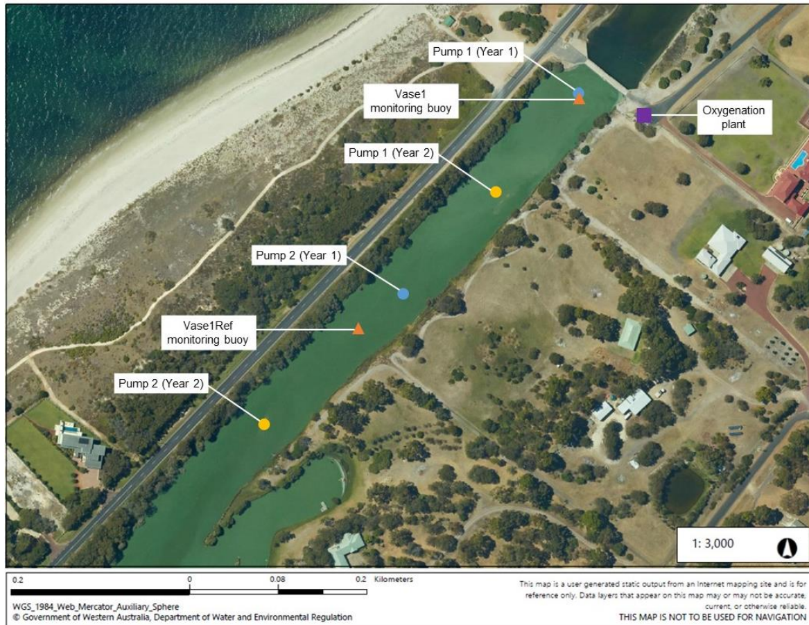
Figure 4 Location of oxygenation plant compound, in-river units and monitoring buoys in both years of the trial
