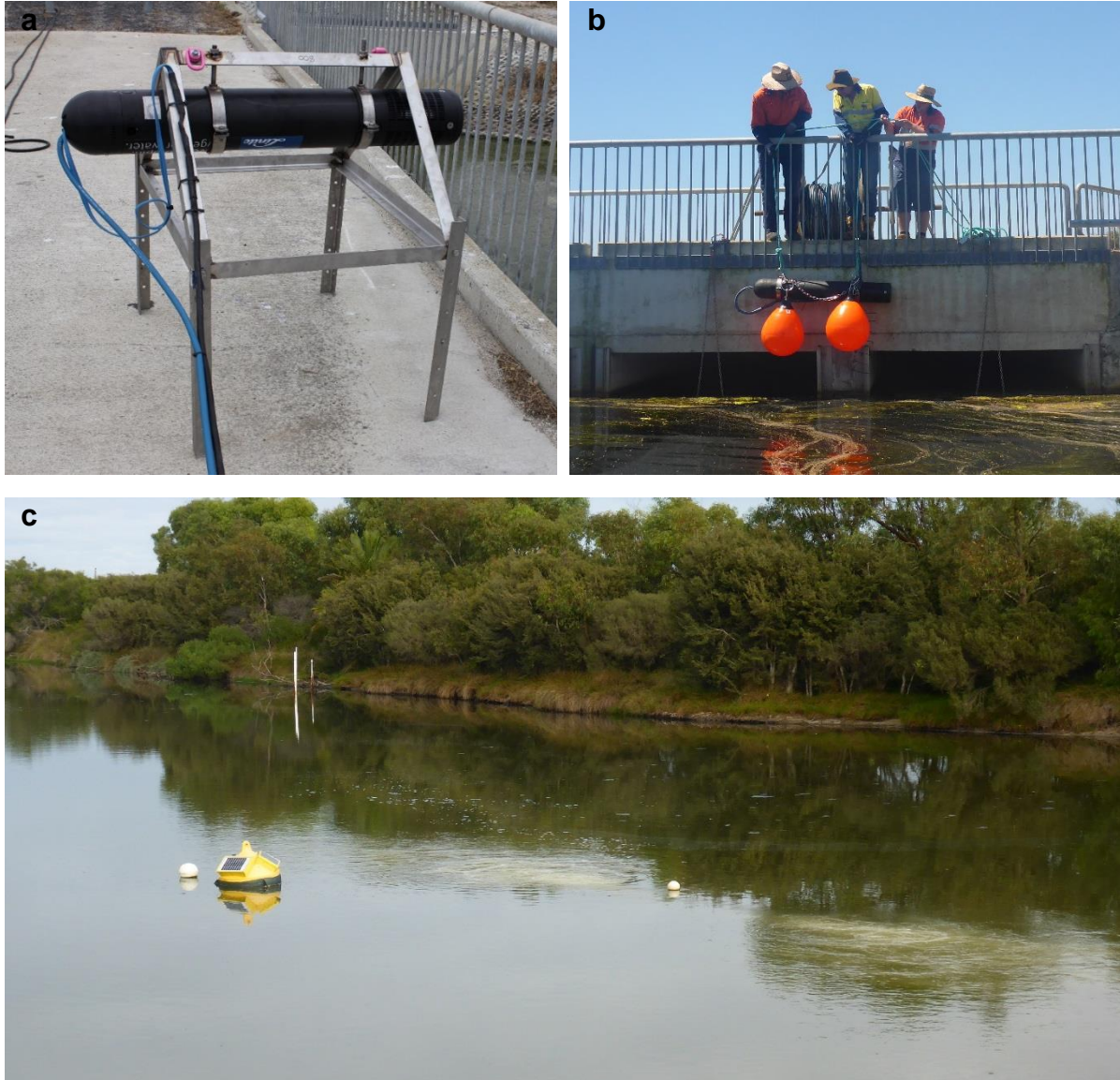
Figure 2 (a) A Solvox drop-in unit mounted on a frame in year 1 of the trial, with oxygen (blue) and electricity (black) supply lines (b) Contractors lowering a unit into the estuary to be suspended in the water column by a buoy in year 2 of the trial (c) The Vase1 monitoring buoy, and the two distinct oxygen plumes of pump 1 in year 1 of the trial.
