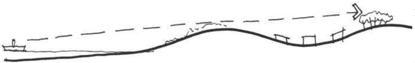
Figure 7: Ensure proposed buildings are hidden between dunes, to maintain a “green” horizon line
