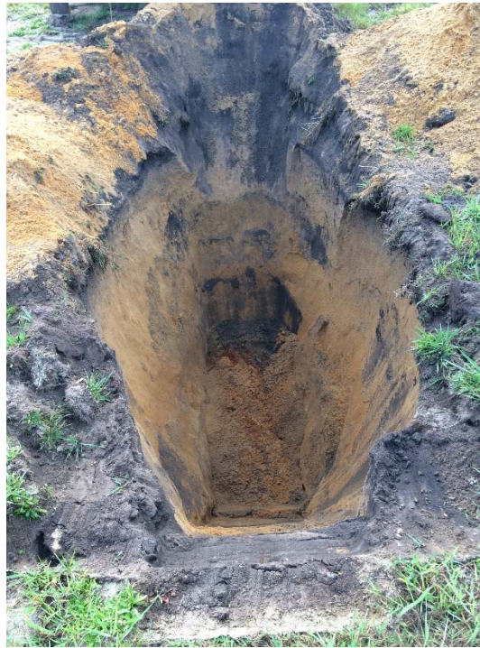
TP04 – TEST PIT EXCAVATION
