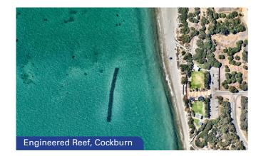
Soft coastal protection options largely include nature based solutions, which aim to mimic natural ecosystems and processes to provide protection. These include works such as sand nourishment, artificial shellfish and coral reefs, revegetation, salt marshes, mangroves and seagrass.
