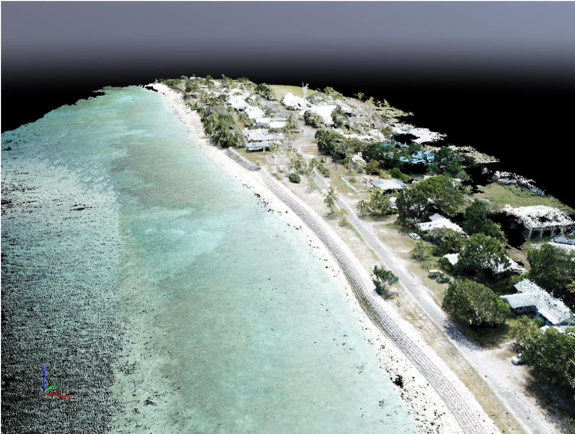
Figure 14: 3D Point cloud of the West Island settlement derived from the July 2018 drone survey using Autodesk Recap Photo.
