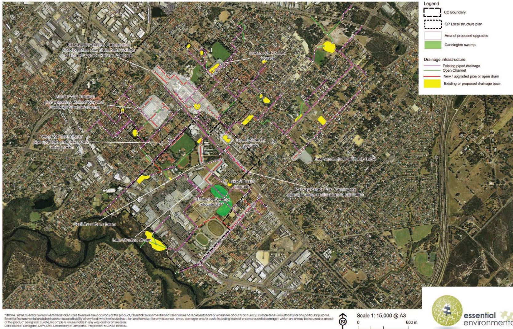
Figure 13.1: Proposed Modifications to Existing Drainage System - Source: CCC Local Drainage Plan, Essential Environment 2016
