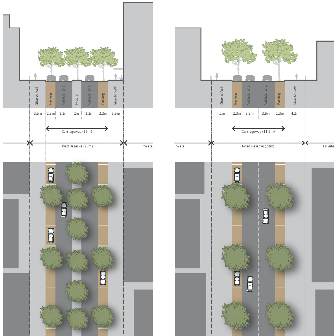
Figure 12.6: Indicative Cross-Sections for Portions of Lake Street, Carousel Road, Pattie Street and Leila Street
