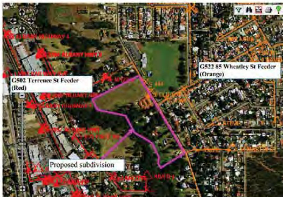
Figure 3 – Existing Power Network
