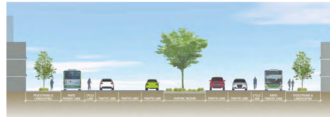
Figure 14 Indicative cross section – Canning Highway
