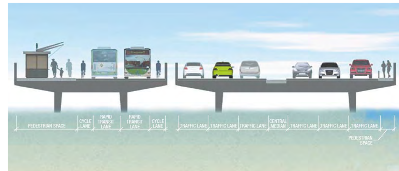
Figure 15 Indicative cross section – Canning River Bridge
