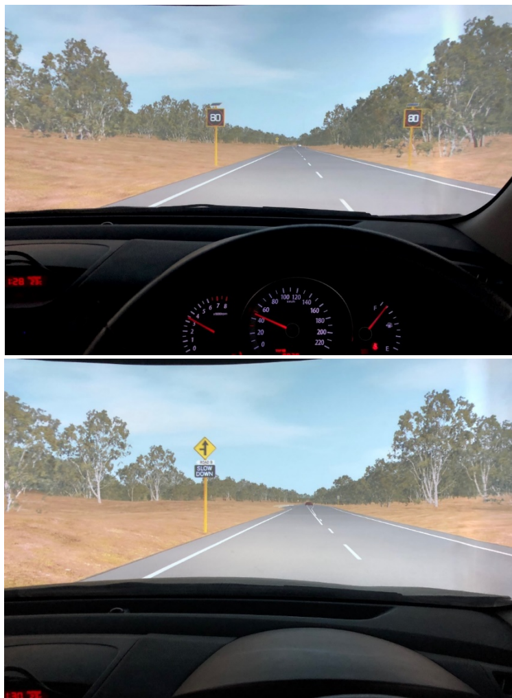
Figure 4.2: Electronic RIAWS 80 km/h speed limit sign and RIAWS slow down sign
