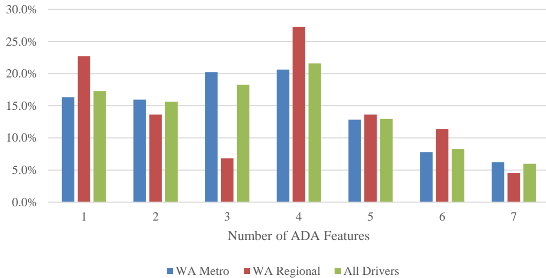
Figure 4.3 Number of Advanced Driver Assist technologies fitted to the car by location
