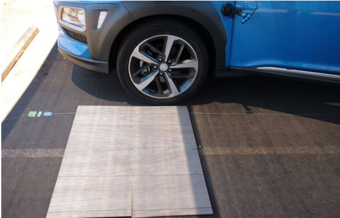
Figure 2.3 Camera overlay being aligned using scale
