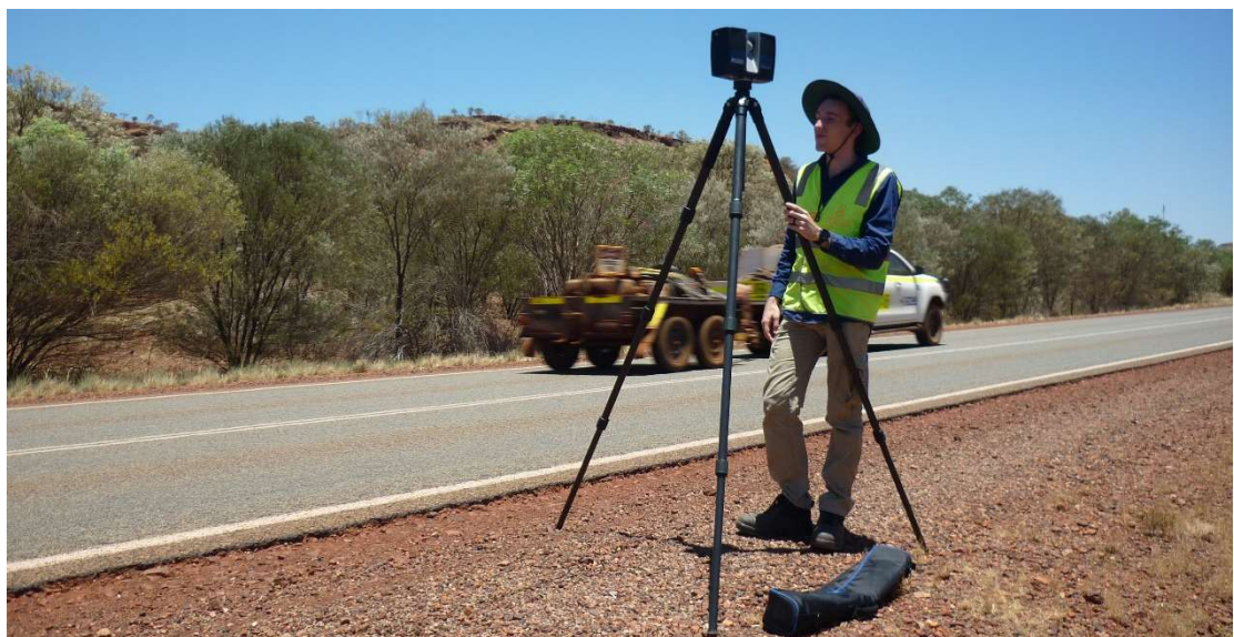
Figure 2.5 Faro S70 Scanner positioned on the side of a road
