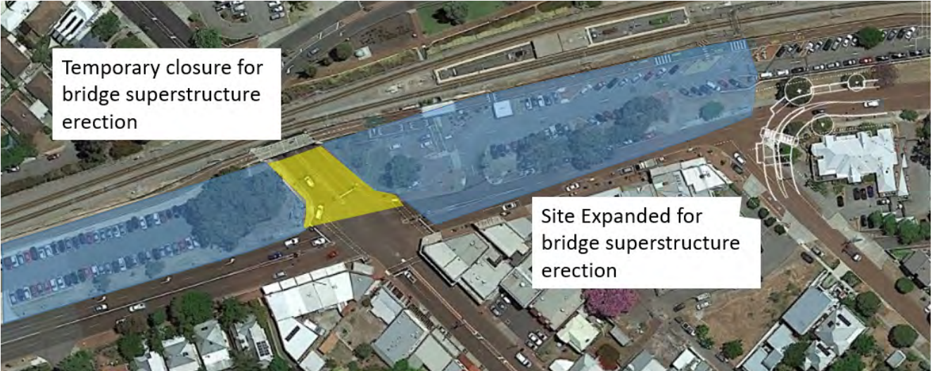
Figure 18.5: Stage 5 – Southern Bridges Superstructure Construction
