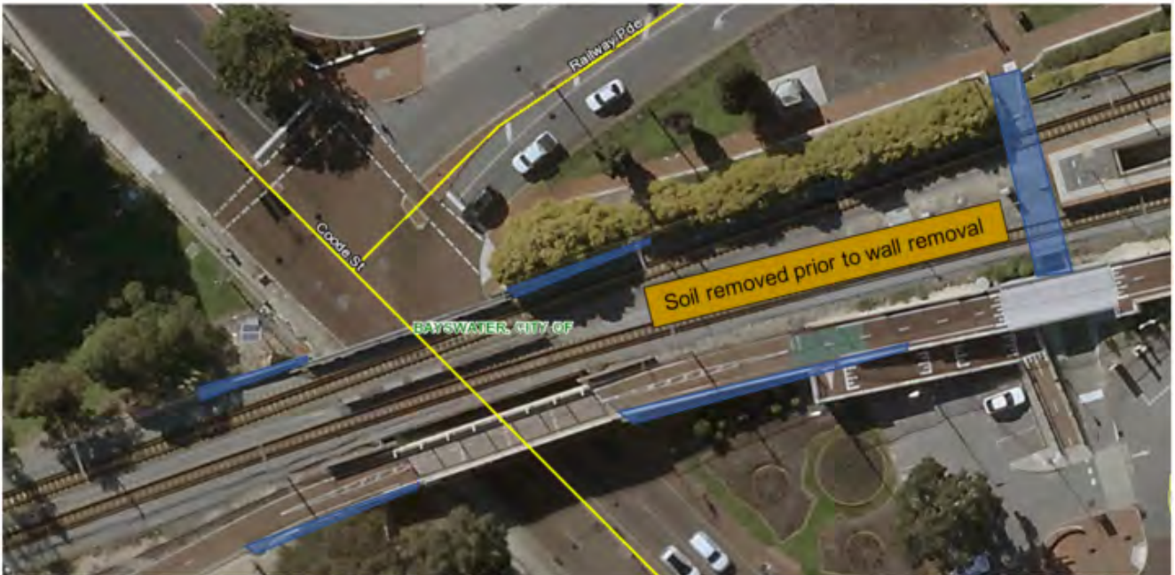
Figure 18.57: Underpass & Wing Walls Demolition
