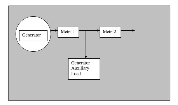
The actual auxiliary load is Meter1 – Meter 2 (from SCADA)
