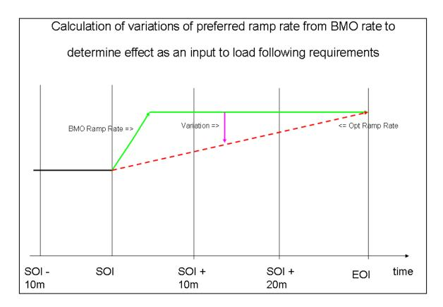
Note that the "BMO Ramp Rate" trajectory starts at the previous EOI target MW not the actual output MW.
