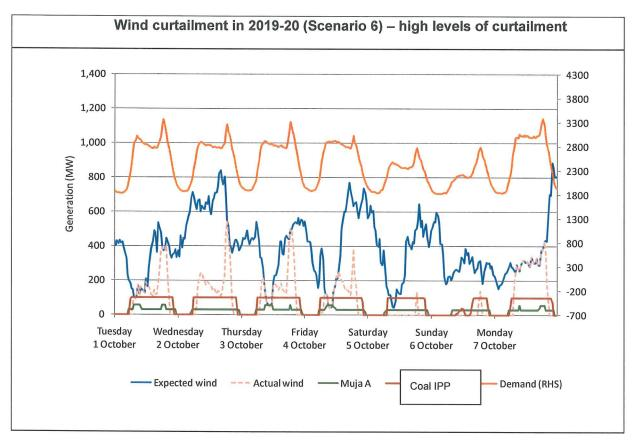
In this scenario, several coal power stations are still required to cycle, despite their mustrun status, during periods of high wind/low demand as shown in the following graph. The large amount of wind combined with the correspondingly large amount of load following gas plant exceeds demand on a regular basis. It should be noted that this degree of cycling, once every day, is infeasible from a Power System Security perspective.
