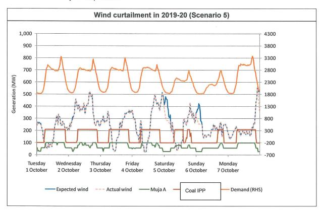
In this scenario, wind is constrained first in every period and therefore lower levels of cycling occur. In scenario 4 (lower wind, lower must-run), by comparison, due to the mix of machines in service, cycling occurs as required and therefore wind output is not curtailed.
