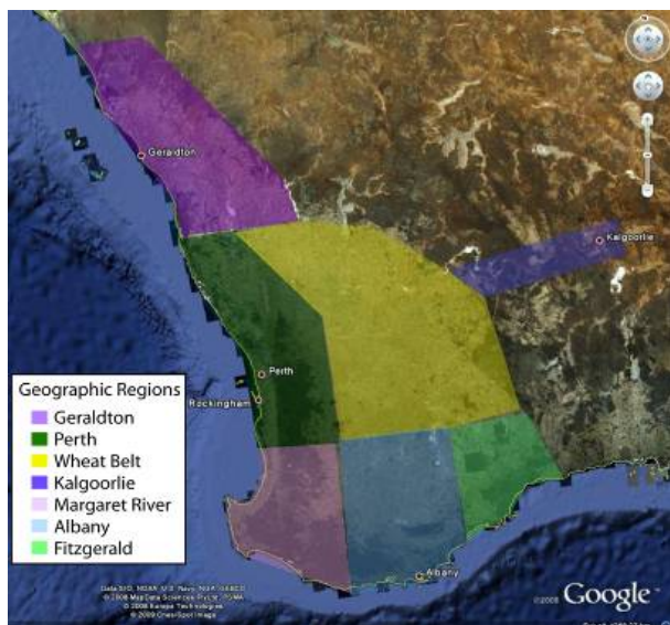
Figure 28: Map showing the approximate boundaries to be used for the fleet calculations. In all there are seven regions considered where each is represented by a single generator from Wind Fleet 2.
