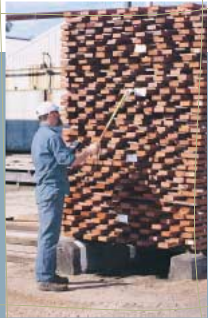
Measuring moisture levels of timber.
