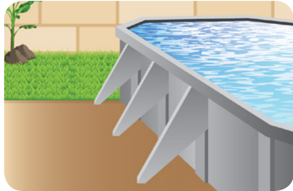
An example of non-climbable swimming pool supports.
