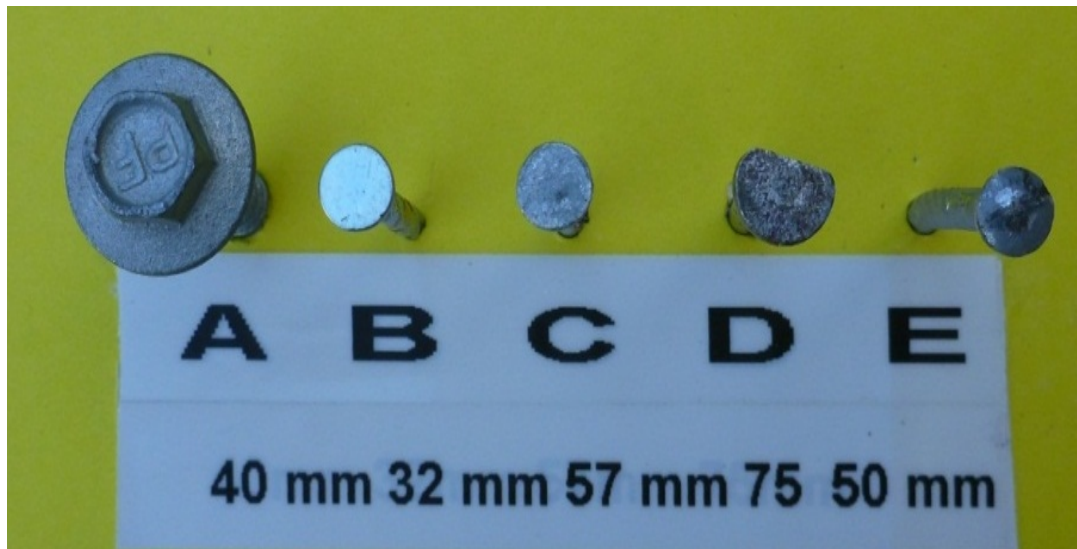
Figure 17. A comparison in the size of the fixing heads between the screw fixings
