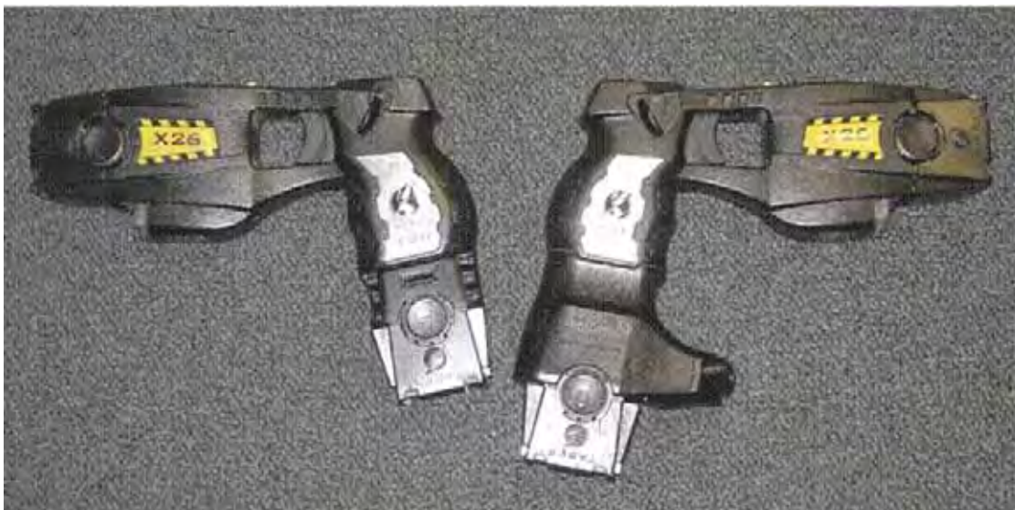
Figure 6: Photograph displaying Taser X26 with spare cartridge attached (left) and spare cartridge and Taser Cam (right)
