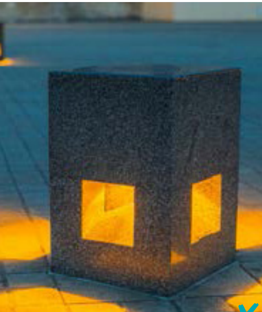
Easily removed or vandalised low-level lighting. ❌
