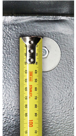
Clearly show the size of the washers by using a ruler or scale
