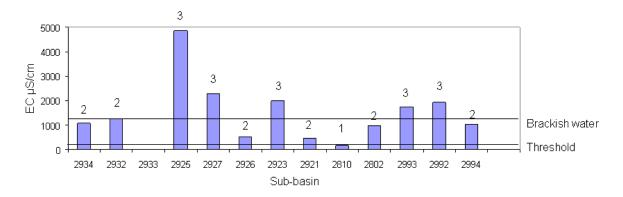
Figure 9 Example of scoring salinity using ANZECC & ARMCANZ (2000) water quality thresholds for tropical rivers for subcatchments along the Fortescue River
