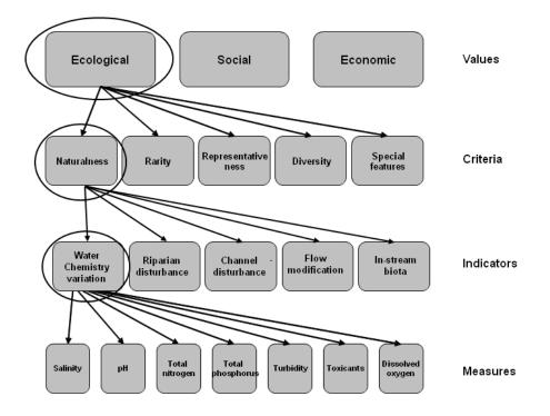
Figure 3 Hierarchy of values, criteria, indicators and measures used to assess the values of waterways in this framework.
